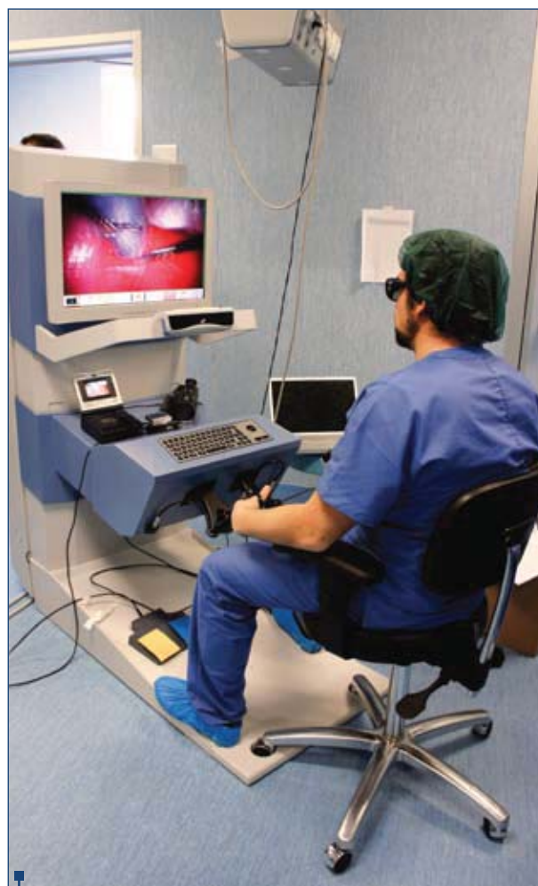
Figure 3. Console with 3D open sight and eye-tracking system
