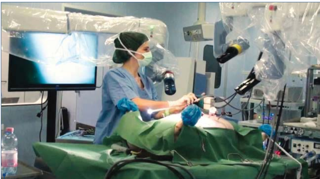
Figure 1. Immediate exchange of instruments, which are attached to the arms with magnets
